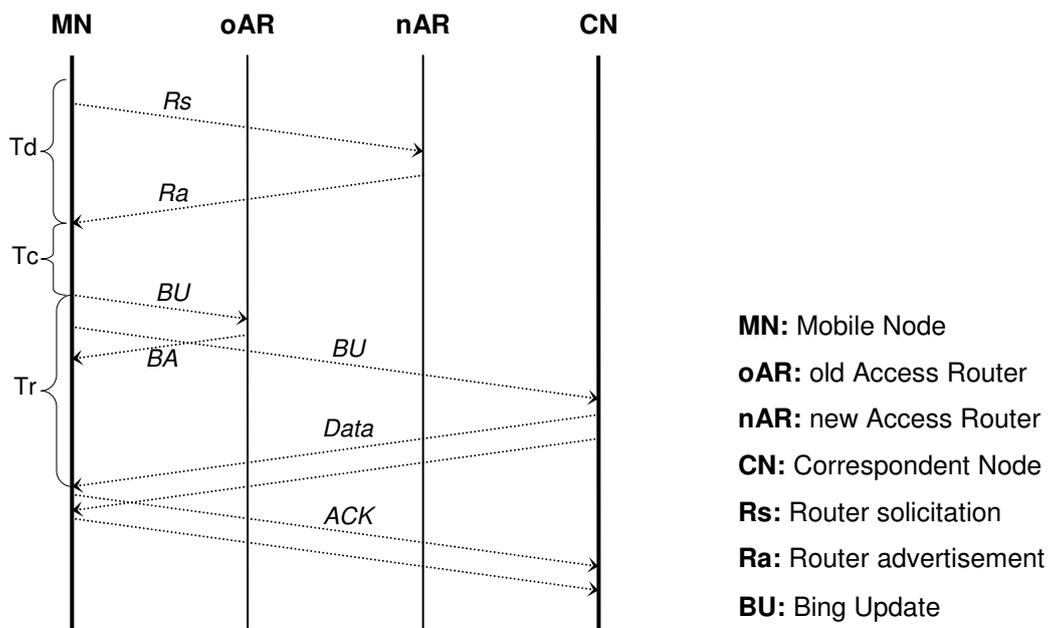
Figure 1: Components of handoff latency in MIPv6
