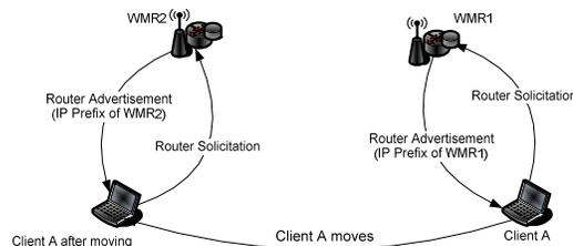
Figure 7: How to get CoA when the mobile client moves to a new domain
