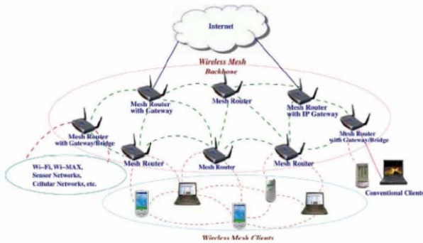
Fig. 3 Hybrid Wireless Mesh Network.
