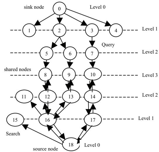
Fig. 7. An example of the double routing trees
