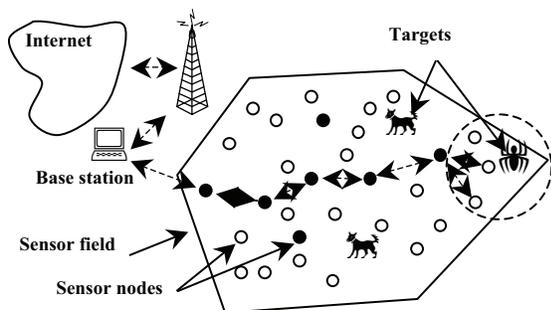
Fig. 1. Communication architecture of a wireless sensor network
