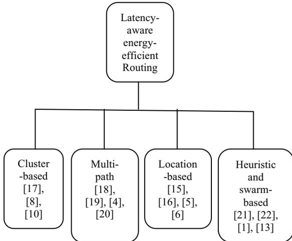
Fig. 2. Classification of Latency-aware energy-efficient routing Techniques in WSNs
