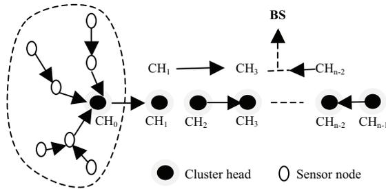
Fig. 5. A combination of cluster and chain scheme
