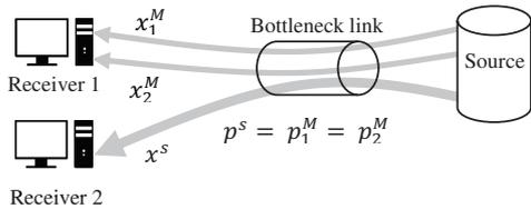
Fig. 1. Sharing bandwidth at a bottleneck link.
