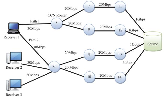
Fig. 4. Simulation topology for congestion balance.
